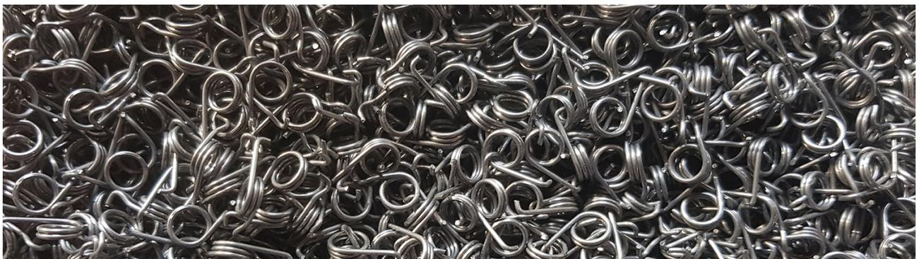
The twin coil torsion springs produced specially for the *smartLock* to my design are precision made and shot-peened - a process used to strengthen and extend the life of high end components used in formula 1 and other high stress environments.
